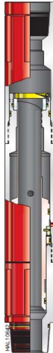
Tubing String Testing (TST) Valve
