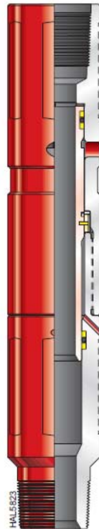
Internal Pressure-Operated (IPO) Circulating Valve
